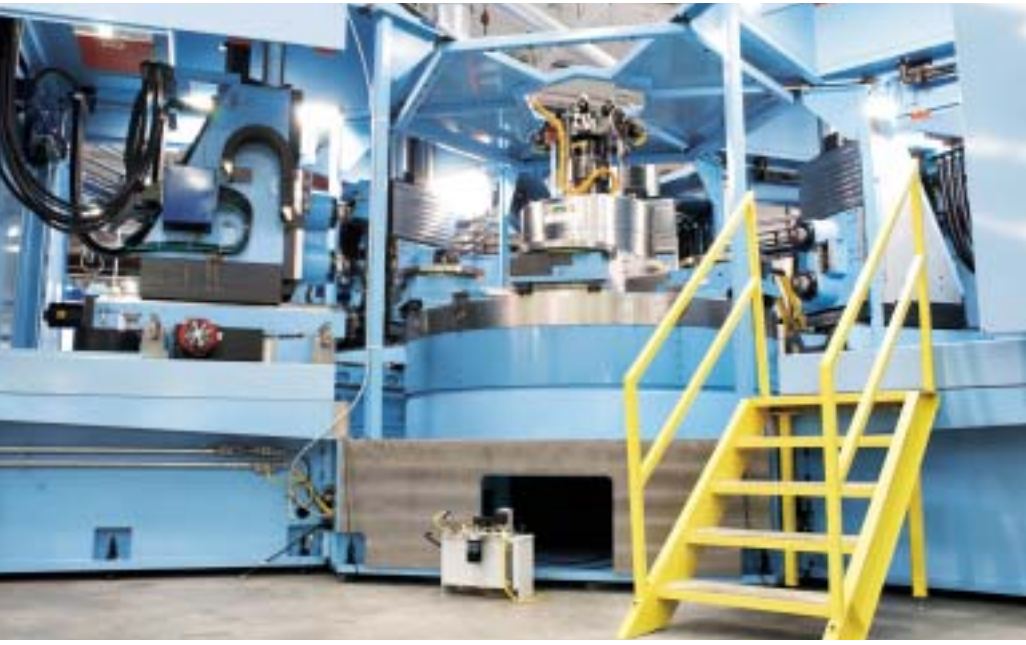
A Liberty rotary-dial machine with twin-spindle three-axis units.
