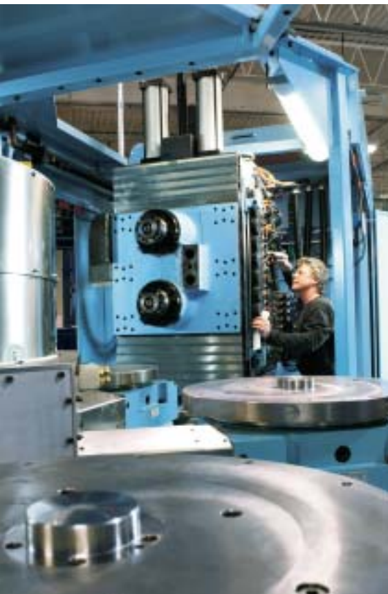
Dennis Kuter works on installing a tool storage rack for the automatic tool changer on a twin-spindle three-axis unit.
